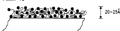
Figure 5. Schematic diagram of physisorbed and chemisorbed PMMA on a surface. Solid dots in the latter case represent sticky side chains containing sulfide groups.
